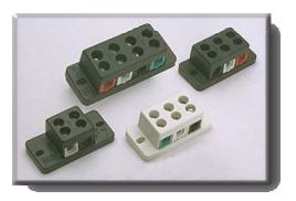
94V-O, 130°C Connector: .0002" (200 micro-inch) thick Matte Tin over Copper Flash over 70/30 Brass Screw: Clear Chromate over .0001" (100 micro-inch) thick Zinc over Steel
